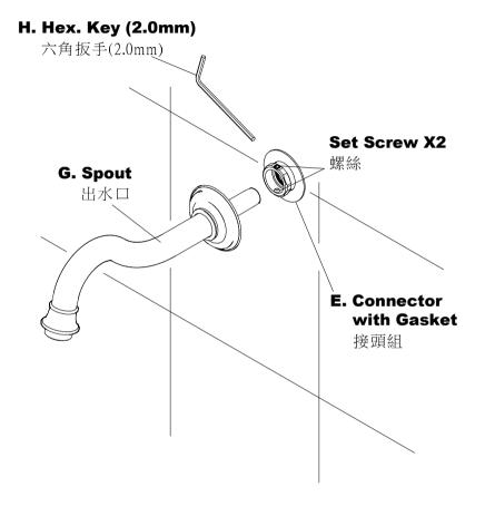
\* Insert the **Spout** into the **Valve Body**, confirm the direction of **Spout**, tighten the **set screws** of **Connector** to fix the **Spout**, and then screw **Flange with O-Ring** to the **Connector**.
