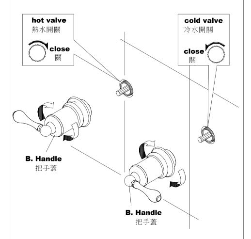
\* Screw the **Handle** to the shanks of **hot and cold valves** till against finished wall.
