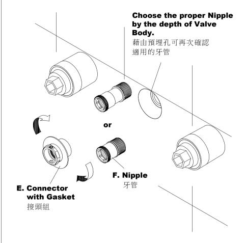
\* Choose proper **Nipple**, apply the pipe compound or thread sealant tape and then screw it to the **Valve Body**. Screw and tighten **Connector with Gasket** to the **Nipple**. In case of forgetting the choosing parts, it could be checked again by the depth of Valve Body.
