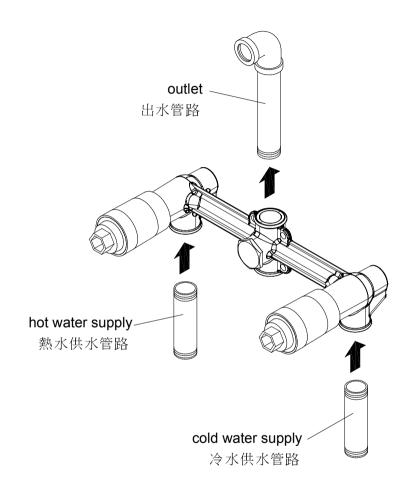
\* Install hot and cold water supply pipes and outlet.
