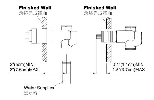
\* Connect hot and cold supply pipes to the **Valve Body**, and keep the distance between 2" (5cm) minimum and 3" (7.6cm) maximum from the Finished Wall to the center of **Valve Body**; or keep the distance be 0.4 " (1.1cm) to 1.5" (3.7cm) between top of cartridge and Finished Wall for necessary conditions.
